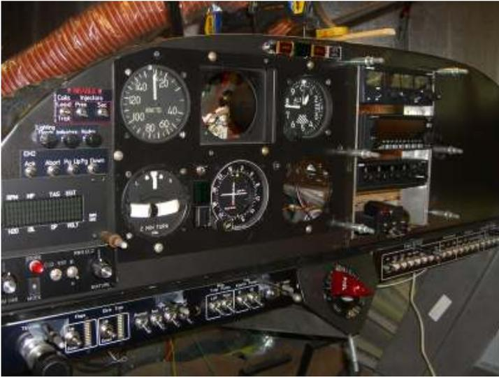
**Scott Stout's Zenith 801 Project:** The past few months have been a lot of work on wiring the instruments and electrical. Instrument and Avionics wiring is complete and electrical wiring in 90% complete. The three electrical buses are completely wired and have passed the all important smoke test on powering up. The three separate buses are divided into flight critical, avionics, and the rest.
