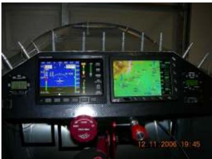
Above are the dual glass displays for Hal Schwab's Sonex - Dynon EFIS and Airmap moving map. Nice "carbon fiber" panel (actually a vinyl stick on!).
