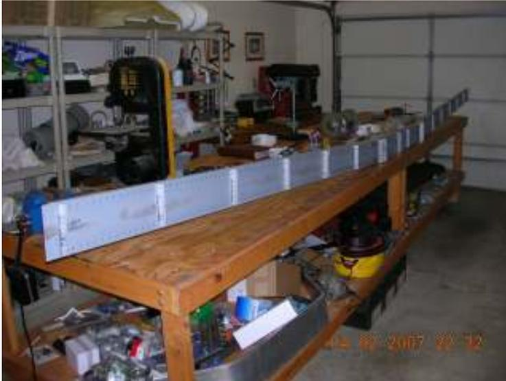
**Bill Wilson** - "Above is a photo of my scratch built center section and wing spars for my **Thatcher CX4**. I had the ribs laser cut, so my next job will be to form the ribs to attach to the wing spars."
