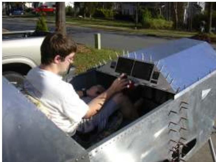
It's starting to look like an airplane! **Hal & Stuart Schwab: Our Sonex** is on its landing gear, the instrument panel is almost done, and we will be rigging the wings in mid December. The tail surfaces have been rigged and drilled, then removed so the plane will fit back in the garage. I would like to cover the instrument panel with a thin carbon fiber veneer. Anyone know where to get some cheap? Y'all come and visit us. You can try the Sonex on for size.
