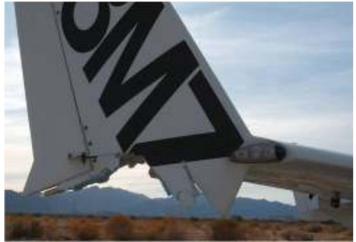
Here's what can happen if you don't regularly check the torque on propeller bolts! However, Craig Catto thinks this was caused by the use of a composite spinner bulkhead.
