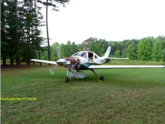
First run fired off on the second blade, but the engine ran rough for the entire 4 minutes. Couldn't get above about 2000 rpm. We ran it three more times to get a feel for why it was choking and limited on the top RPM. The problem was illuminated by abnormally low fuel flows as evidenced by the fuel pressure readings on the EFIS. Dennis Hallman had a couple of ideas, as did Andy and our own thoughts. The flow tests of the aircraft fuel system later in the day were good - close to 60 gal/hour.
